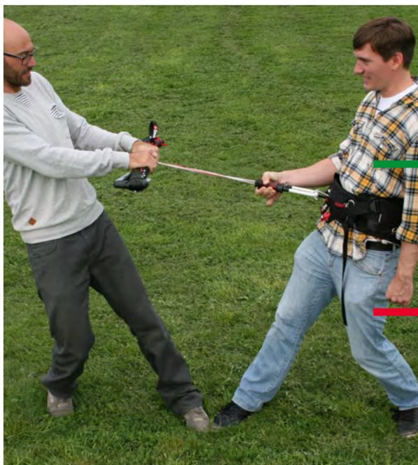
In order to effectively test your Quick Release, it is important to try **releasing it under load**. Ask a friend or colleague to help you as shown on the picture. Try to apply a load of at least 15 kg. A release test without load on the system is not sufficient.
